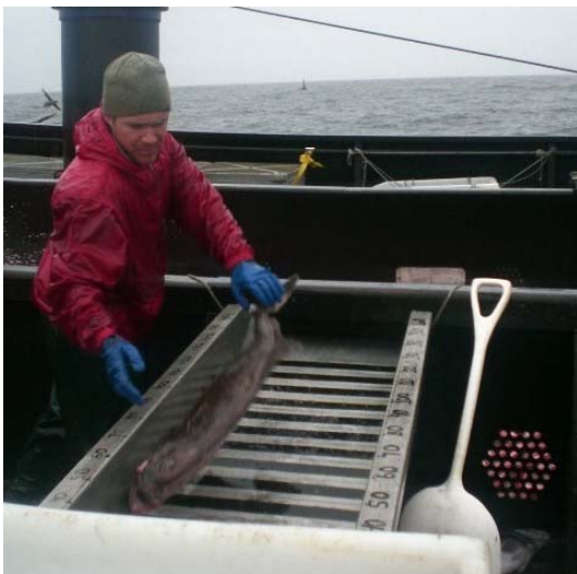
Figure 1. Discard chute for recording halibut discards showing the grid system for calibrating fish lengths.
