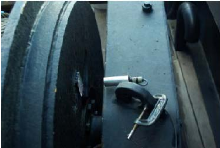
Figure A5. Drum rotation sensor mounted on trawl warp winch, showing optical sensor and reflective surface.
